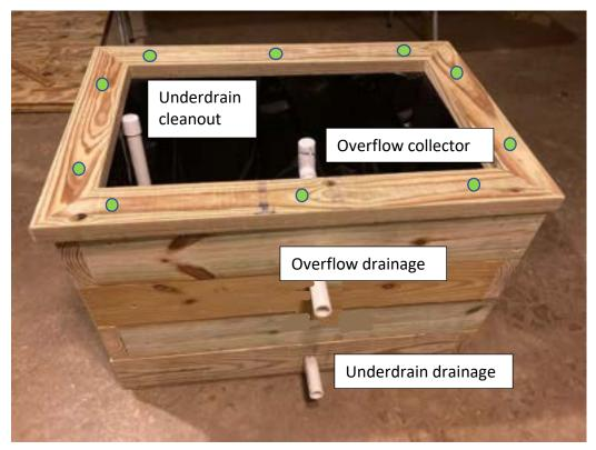
Cement two 7" pipes to each bulkhead and through the planter holes to act as drainage for the underdrain and overflow.
