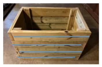
Continue stacking and using two screws to affix 2x6 ends to each other, alternating the position of the end boards as shown in the picture to the left.
